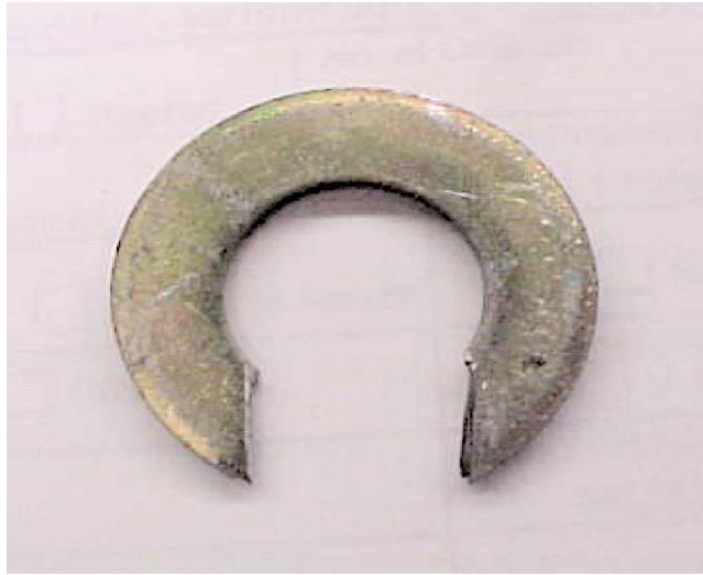
Figure 14 Illustration of Shim Fabricated From P/N D8400-7936 Washer
